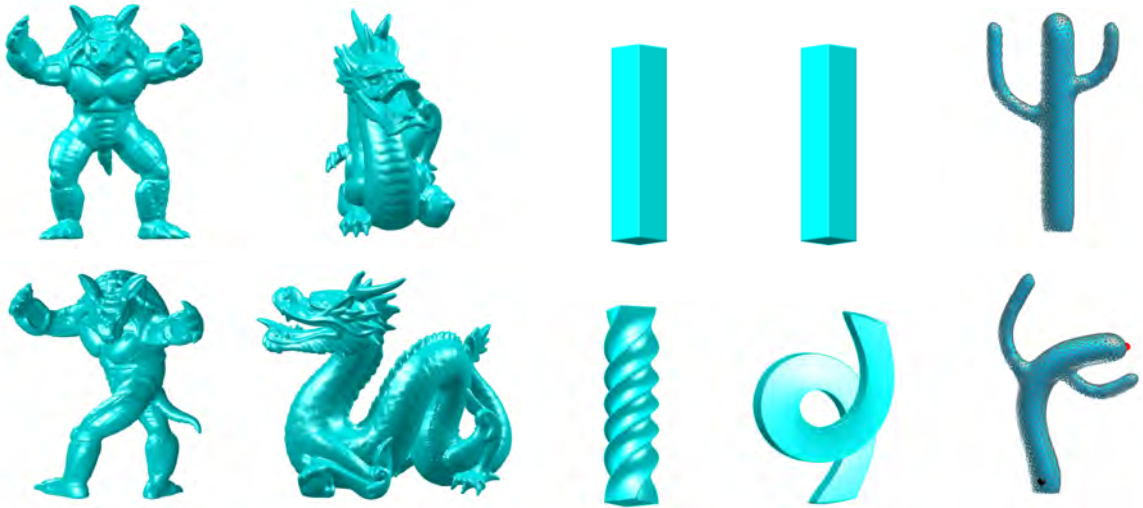
Figure 3.8: Deformation on Armadillo, Dragon, Bar & Cactus mesh. (Row 1) Original meshes, (Row 2) Deformed meshes. For Armadillo, 3 handles (one on each foot, one on the forehead) are used and deformation is achieved by rotating the handle on the forehead by 180 deg. We use 4 handles for the Dragon mesh to generate the large deformation. For the Bar mesh, results of applying rotations by 3\pi and 2\pi (col. 3 and 4) using only two handles (one on top and one on bottom) are shown, while the Cactus mesh is bent by 60 deg using 5 handles.
