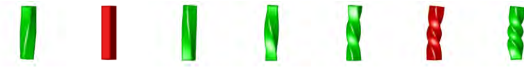
Figure 5.1: Twisting of a bar - An example of Interpolation and Extrapolation. From left to right, the meshes correspond to time t = -.25, 0, .25, .5, .75, 1, 1.25 , where mesh at t = 0 corresponds to the initial mesh and mesh at t = 1 corresponds to the final mesh. Note that without the proposed segmentation based interpolation approach, this particular large deformation interpolation example will not produce intuitive results. Also, note that our approach is able to extrapolate the deformation.
