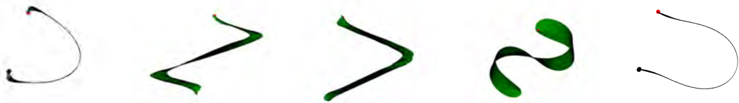
Figure 3.10: Cigar one-step deformation by rotating the moving handle out of the plane by an angle of 144 deg. (left to right) LRI, FAST, LS-ARAP, SR-ARAP, Proposed. While LRI produce intuitive results, FAST, LS-ARAP and SR-ARAP twists the cigar. The proposed algorithm yields intuitive results and does not vary with the amount of deformation. Results for FAST and LS-ARAP are computed with 80 auxiliary handles.
