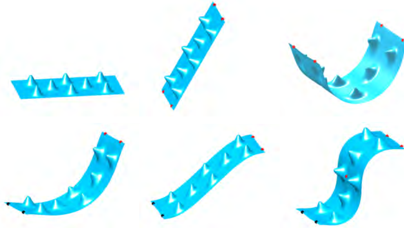
Figure 3.13: (Clockwise from top left.) (a) Original Mesh (b) Global rotation using both, handle translation and rotation, (c) Bending using handle rotations, (d) Lifting from a side using fixed handles and handle translations and rotations, (e) Lifting from a side using fixed handles and handle translations only, (f) Realistic lifting from a side using combination of fixed handles, handle rotations and translations, with 2 additional handles.
