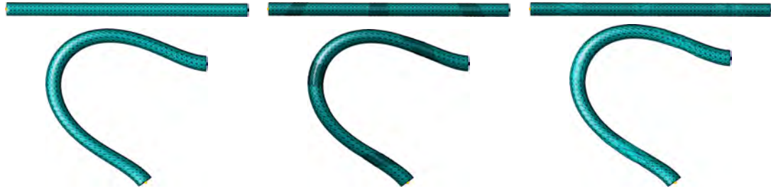
Figure 3.14: Effect of change in resolution. Row 1 shows original meshes, while Row 2 provides deformed meshes obtained via same handle deformations. The number of handles used is 2, shown in yellow (moving) and black (fixed). The left column demonstrates the deformation on the original cylinder mesh, while the center and right column demonstrates the deformation for the mesh with larger and smaller resolution in selected areas, respectively. The number of vertices and faces in these meshes from left to right is (1212, 2420) , (2022, 4036) , (997, 1990) .
