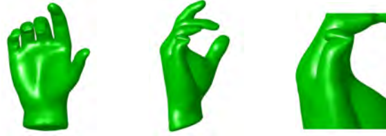
Figure 5.3: Incorrect direction of bending of the little finger due to large deformation between source and target hand meshes. The source and target mesh are the same as used in Figure 5.7. Front-view(left), side-view(center), and close-up of the little finger, of the interpolation result at time t = 0.5 .
