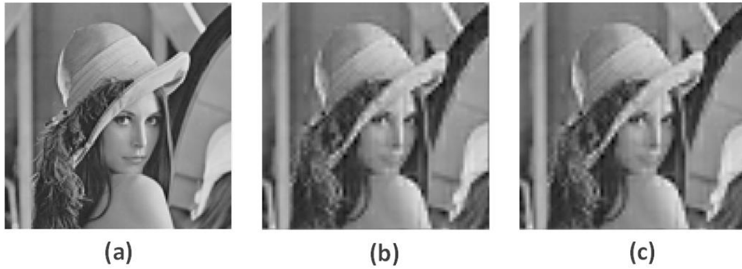
Figure 5.23: DWT Results on 128 \times 128 Lena intensity image (a) Actual (b) MATLAB simulated (c) Hardware computed.
