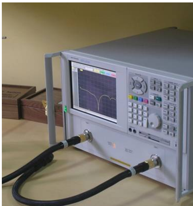
Figure A.1: Agilent Technologies: N5230A (10 MHz to 50 GHz), PNA series vector network analyzer
