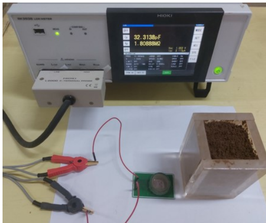
(d) Sensor deploy in soil sample connected with LCR meter
