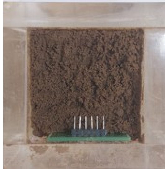
(b) Soil sample in mold mad GO sensor deploy in a soil sample
