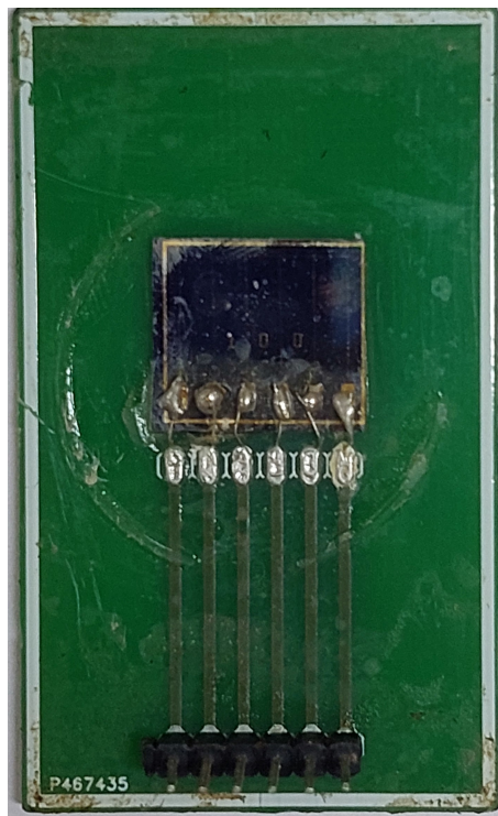
(a) Si wafer placed on PCB and pull out a wire from Si wafer to PCB
