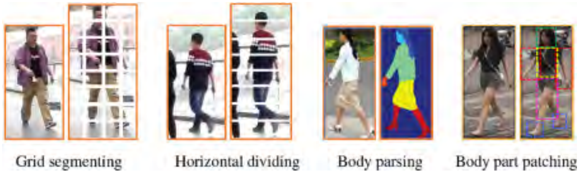
Figure 1.4: Various types of patch-wise data processing techniques to get the local representations of the different features [1]
